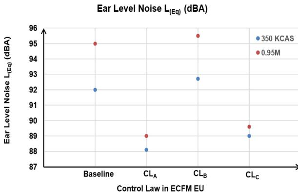
Fig. 7: Ear Level Noise Recorded at  $Z_p=5100\text{ft}$  at 350 KCAS and 0.95M
