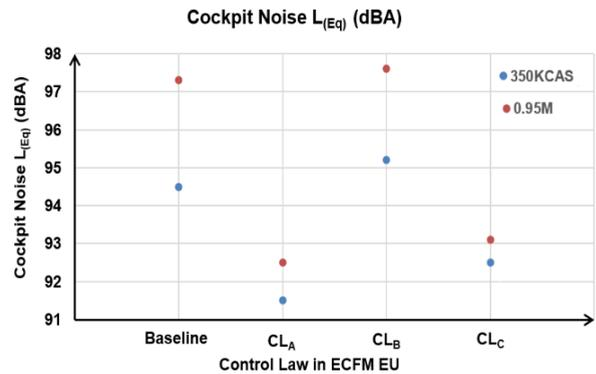
Fig. 9: Cockpit Noise Recorded at  $Z_p=8600\text{ft}$  at 350 KCAS and 0.95M
