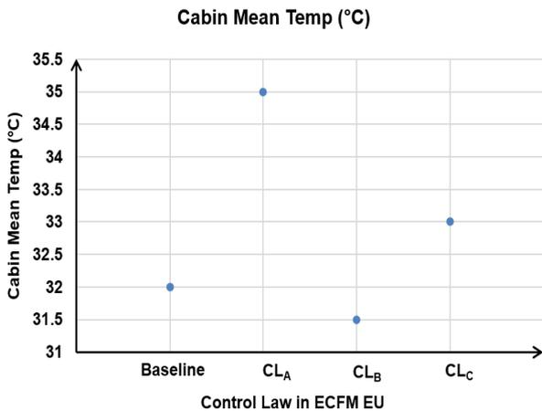
Fig.5: Mean Cabin Temperature Recorded at Zp=3000ft
