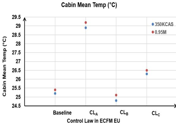
Fig. 8: Cabin Mean Temperature Recorded at  $Z_p=5100\text{ft}$  at 350 KCAS and 0.95M
