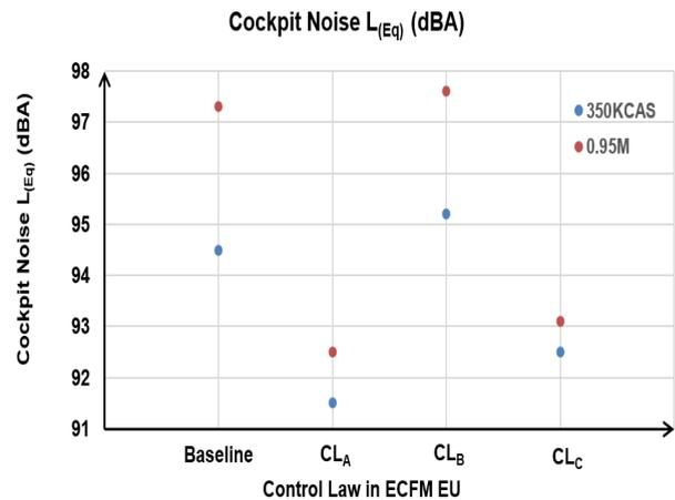
Fig. 6: Cockpit Noise Recorded at Zp=5100ft at 350 KCAS and 0.95M
