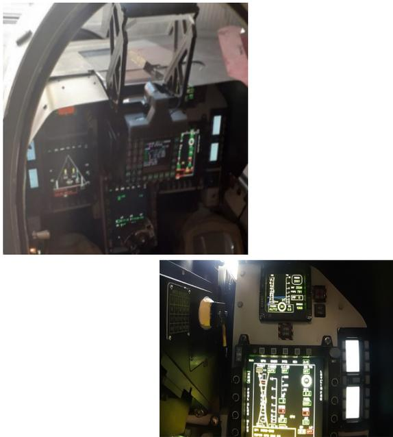
Fig. 2: Photograph of the EFI Display in the Cockpit for Control Law Selection by the Pilot
