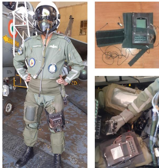
Fig. 1: Photograph of Test Pilot Wearing Helmet along with Recording Equipment
