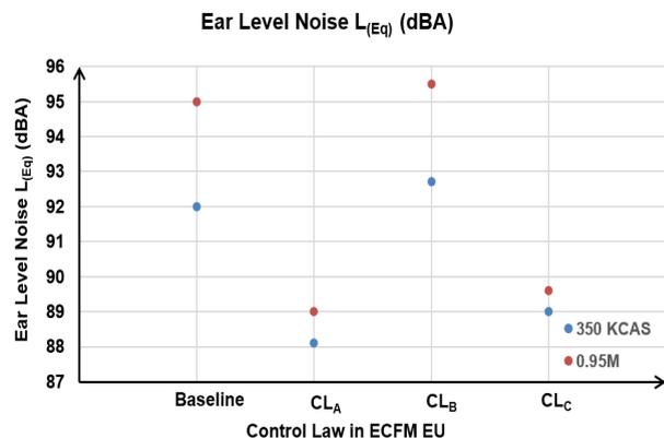
Fig. 10: Ear Level Noise Recorded at  $Z_p=8600\text{ft}$  at 350 KCAS and 0.95M
