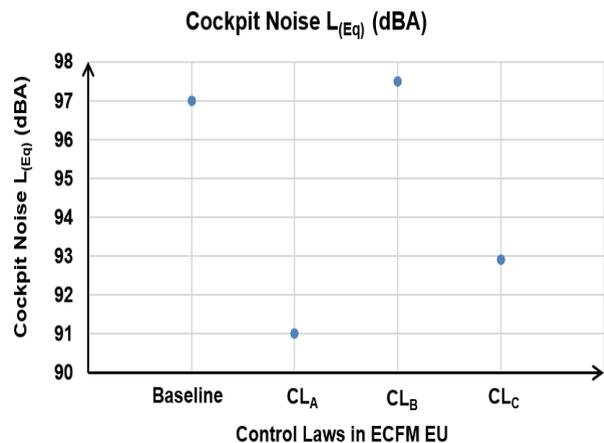
Fig.3: Cockpit Noise Recorded at Zp=3000ft
