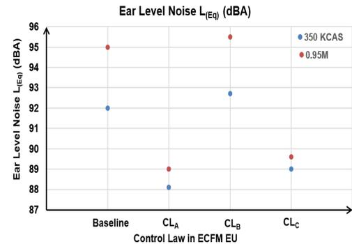
Fig. 13: Cockpit Noise Recorded at Zp=15100ft at 350 KCAS and 0.95M
