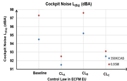
Fig. 12: Cockpit Noise Recorded at Zp=15100ft at 350 KCAS and 0.95M
