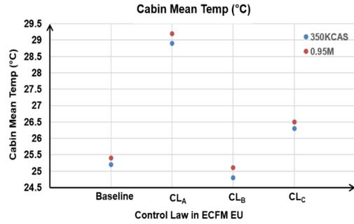
Fig.11: Cabin Mean Temperature Recorded at Zp=8600ft at 350 KCAS and 0.95M
