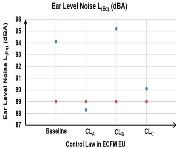
Fig. 4; Ear Level Noise Recorded at Zp=3000ft
